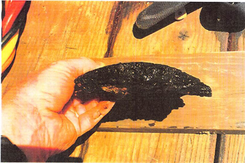
Figure 9: Typical Profile of Dislodged Internal Buildup
